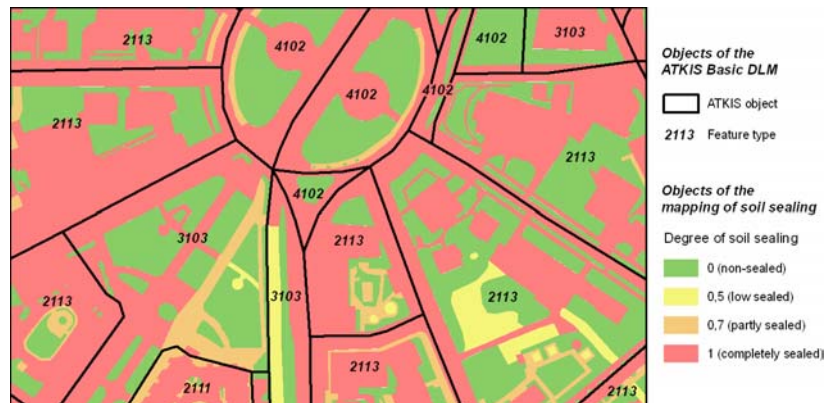
Fig. 1: soil sealing mapping (reference) overlaid with the boundaries of the ATKIS basic DLM (part of the city centre Dresden)
