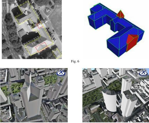
Fig. 7 Visualisation of reconstructed buildings from LiDAR data
