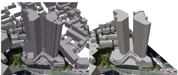
Fig. 8 Rectangle Segmentation (left) and Cell Decomposition (right)
