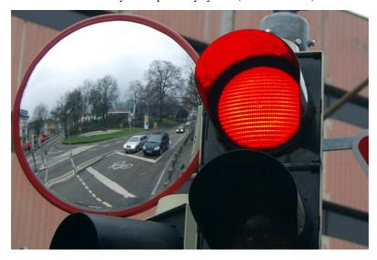
Fig. 7. "Trixi Spiegel" mirror which allows truck drivers to observe cyclist riding parallel (Photo: M. Beim)
