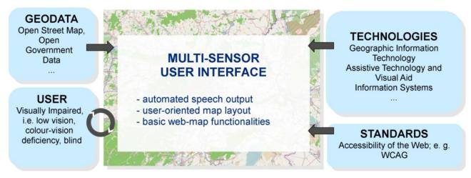
Fig. 3: Components of the AccessibleMap application.
