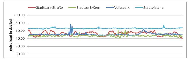
Fig. 3: Comparison of the noise levels from the 4 study locations (Own figure, based on work of Diehl, Michel and Keller for the study project Sensing the City, 2012)
