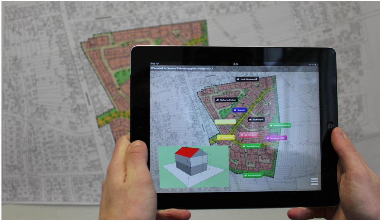
Fig. 8: Marker-based AR-Visualization of a development plan with building codes (Zeile 2011)
