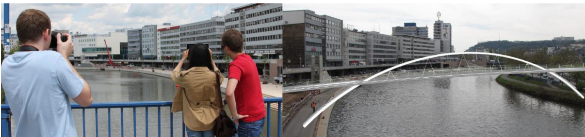
Fig. 3: Use of Augmented Reality to overlay the new virtual design of a pedestrian bridge over the real picture- (Research Group CPE)
