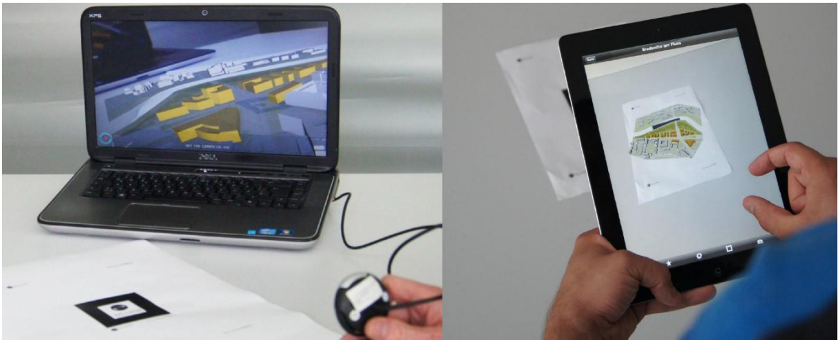
Fig. 4: Visualization of a new design in AR Media, (left) Visualization over Webcam and Notebook, (right) iPad (Research Group CPE)
