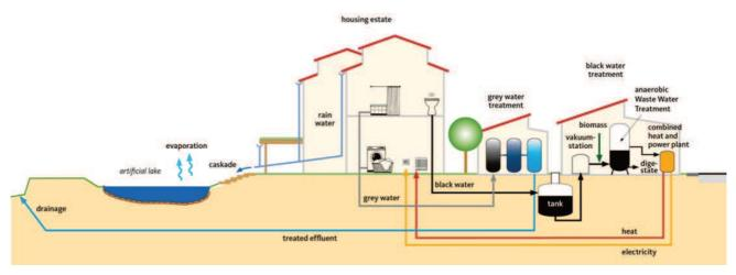
Fig. 8: Separate treatment of storm-, grey- and black water in the new settlement Hamburg Jenfelder Au. Source: Hamburg Water Cycle
