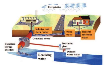
Fig. 5: Combined sewer system under rainy conditions (modified after: Lehn 2002).
