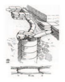
Fig. 3: Waste water disposal into the underground in Assur (Mesopotamia) 2.500 BC (Source: Illi 1987).
