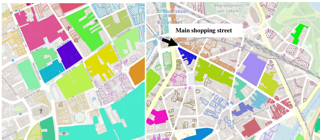
Figure 2: Distance clusters with ST_Cluster_Within at 0,1m (full colour polygons), 20m (striped polygons) and 100m (dotted polygons). Left: Inner city with primary and secondary shopping street in Roeselare, Flanders: At 0,1m distance, it is logical that roads slice groups that should be together. However, from an spatial economic perspective this does not make sense. Right: A main shopping street in Brussels outer city centre is sliced into several groups. (Background layer: Open Street Map)
