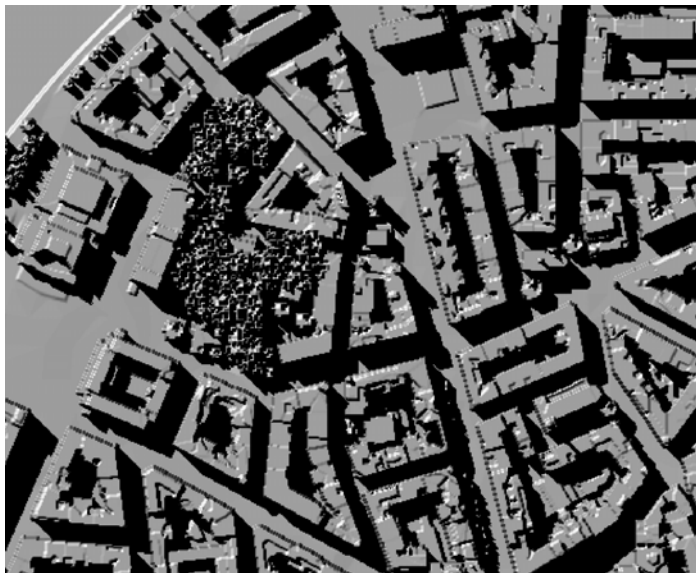
fig. 6: Detail of 1m hillshade grid with shadow rendering
