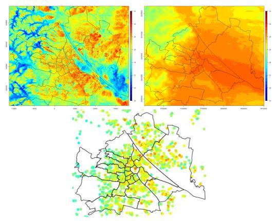
Fig. 1: Air temperature (°C) in Vienna on 16. August 2022 at 19:00 UTC calculated by PALM-4U model (top left), MUKLIMO\_3 model (top right) and derived from quality-controlled monitoring dataset of NETATMO private weather stations (bottom).
