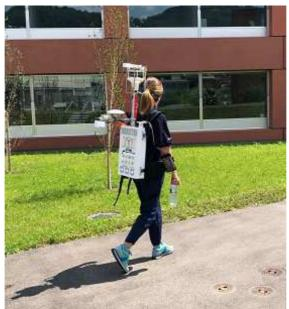
Fig. 6: the measurement campaign in Mendrisio (CH) with the HEPIA Climameter. Elaborations by the authors (2023).
