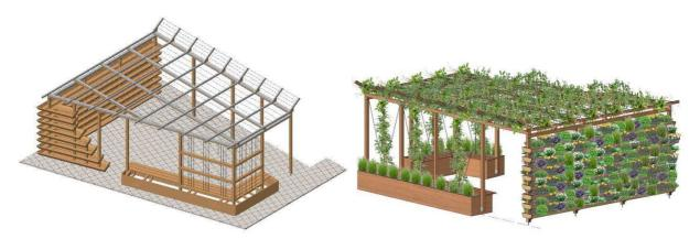
Fig. 6 and 7: Construction details and visualisation of a draft of the outdoor classroom with EVAPO+ transpiring green wall
