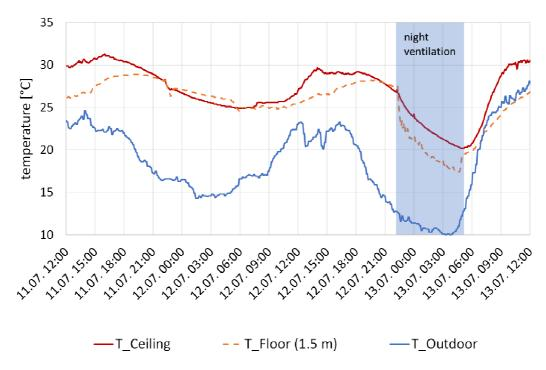
Fig. 3: Effects of the night ventilation test by using the fire ventilation system.
